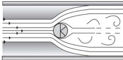
The square sensor profile with its well defined 'edges' and external plenum tubes produces a fixed fluid separation point for all liquids and gases ensuring optimum accuracy independent of Reynolds Number and flow rate.
