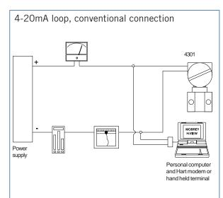
The HART interface is optional and only required for complex, remote configuration. Local, external zero and span adjustment is standard.
