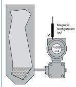
Zero pressure is applied, magnetic tool inserted into 'Z' hole, transmitter is zeroed.
