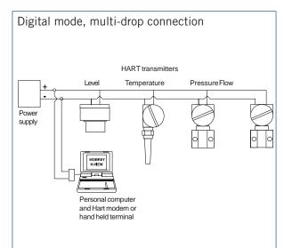
The 4301 may be configured as a controller and connected via the multi-drop technique whilst retaining the 4-20mA output. (Request technical data sheet TD020)
