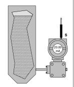
Span pressure is applied, magnetic tool inserted into 'S' hole, transmitter is now calibrated.
